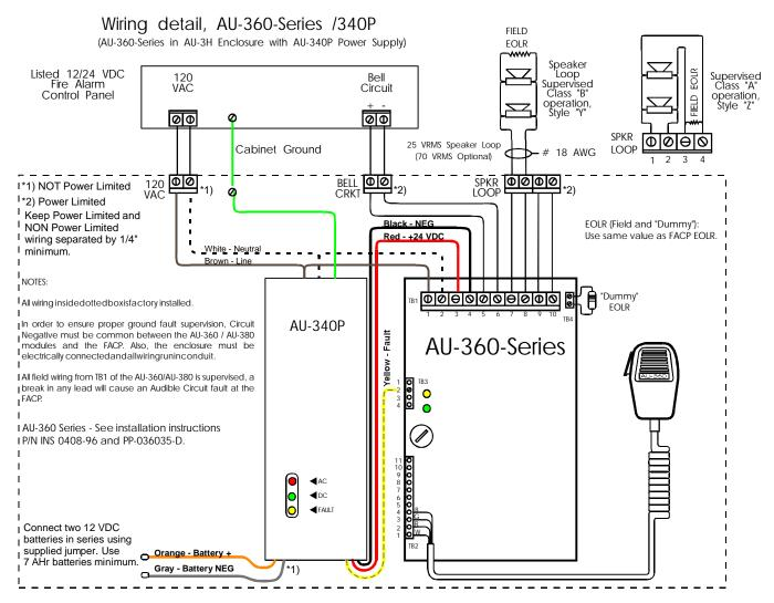
When operating from batteries, the AU-340P and the AU-360/AU-380 enter a battery saver mode. In this mode, the AU-340P draws 10 mA and the AU-360/AU-380 will draw either 6 mA or 18 mA, respectively. This adds up to a maximum of 28 mA for standby on batteries. The AU-380 draws 3.0 A when in alarm with a full 40 Watts of load on the Speaker Loops. This is full power operation.
